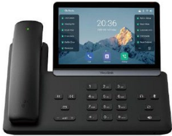
Yealink SIP-T88W – W PRO – V PRO 7" adjustable touch-screen, WiFi, Bluetooth, Up to 84 programmable keys, 2 USB 2.0 ports, opt wireless handset, opt camera, up to 3 EXP55
