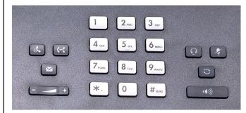
The + and - buttons below the 4-way keypad adjust the volume. Pressing these keys when you are not engaged in a call adjusts the ringer volume. Pressing them while you are in a call adjusts the volume of the handset, speaker, or headset.
