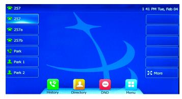
The keys along the side of the screen are programmable, and change depending on the configuration of your phone. In this example, there are three line keys and three park buttons. The keys on the right side have not been programmed, so they are blank. The bottom right "More" softkey displays 18 additional softkeys in the center part of the screen.
