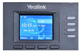
The keys on the side of the screen are programmable, and change depending on the configuration of your phone. In this example, there are two line keys on the top two buttons.
