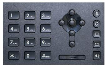
The four-way keypad is used to navigate the phone's menu system, and the four keys also double as shortcuts. Pressing UP displays the call history, and pressing DOWN displays the number directory, LEFT and RIGHT select the line appearance key to use for making an outgoing call.
